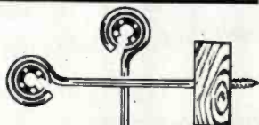
It's a machine screw insulator
